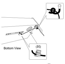
4. Insert the pedal connection cord that comes from Pedal Board (C) into the piano's pedal jack and fasten with cord clamps.
